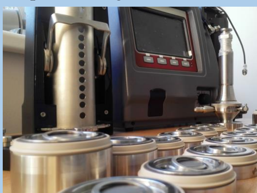
Figure 2. PM 0.1-10 size, mass and number distribution detection by ELPI+, Dekati.
